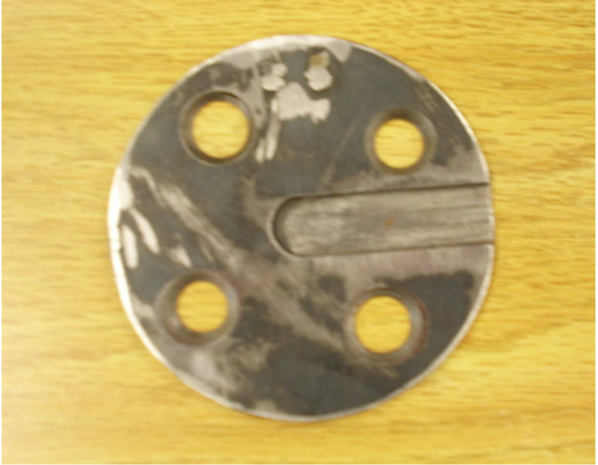
Figure 4.1. Picture of bottom fixation device used in setup for testing in shear.
